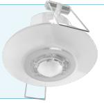
This passive infrared motion detector can be installed into any ceiling to control individual or groups of fixtures. It functions as both an occupancy and vacancy sensor and also acts as a daylight harvester.
